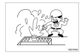
Do not work below the machine. Be sure to work with proper safety supports.
