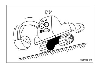
Avoid parking and stopping on a slope. Lower the bucket to the ground and block the track when parking.
